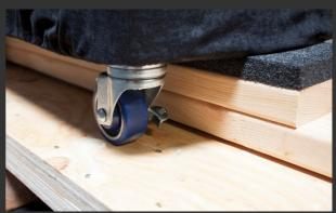
With one person on either side of the crate walls, lift straight up and backwards, removing the walls of the crate. Set walls aside. The speaker will be sitting free on the base. Disengage the brakes on the casters; position the casters parallel to the ramp and facing the back of the crate for smooth removal.
